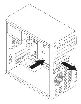
Figure 26. Removing the diskette drive or card reader
